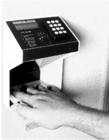
Figure 3: Access control device using hand geometry for identification
