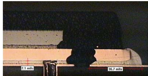
81% Paste Coverage, Encroached Via, 2.1 mil Standoff
