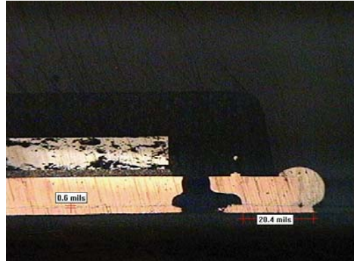
37% Paste coverage, Encroached Via, 0.6 mil Standoff
